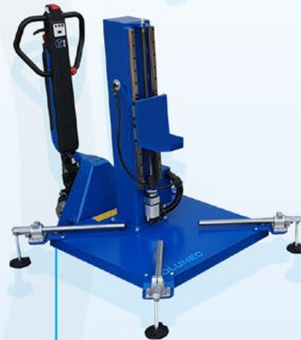
CSM002-2WD: TROLLEY WITH ADJUSTABLE LIFTING COLUMN. Electric motorized trolley. Column H= 1060 mm and stroke 600mm. Handling through brushless motor 400W – 220 V. Piloting by electronic accelerator and up and down buttons. Total weight 480 kg (1058 lb).
